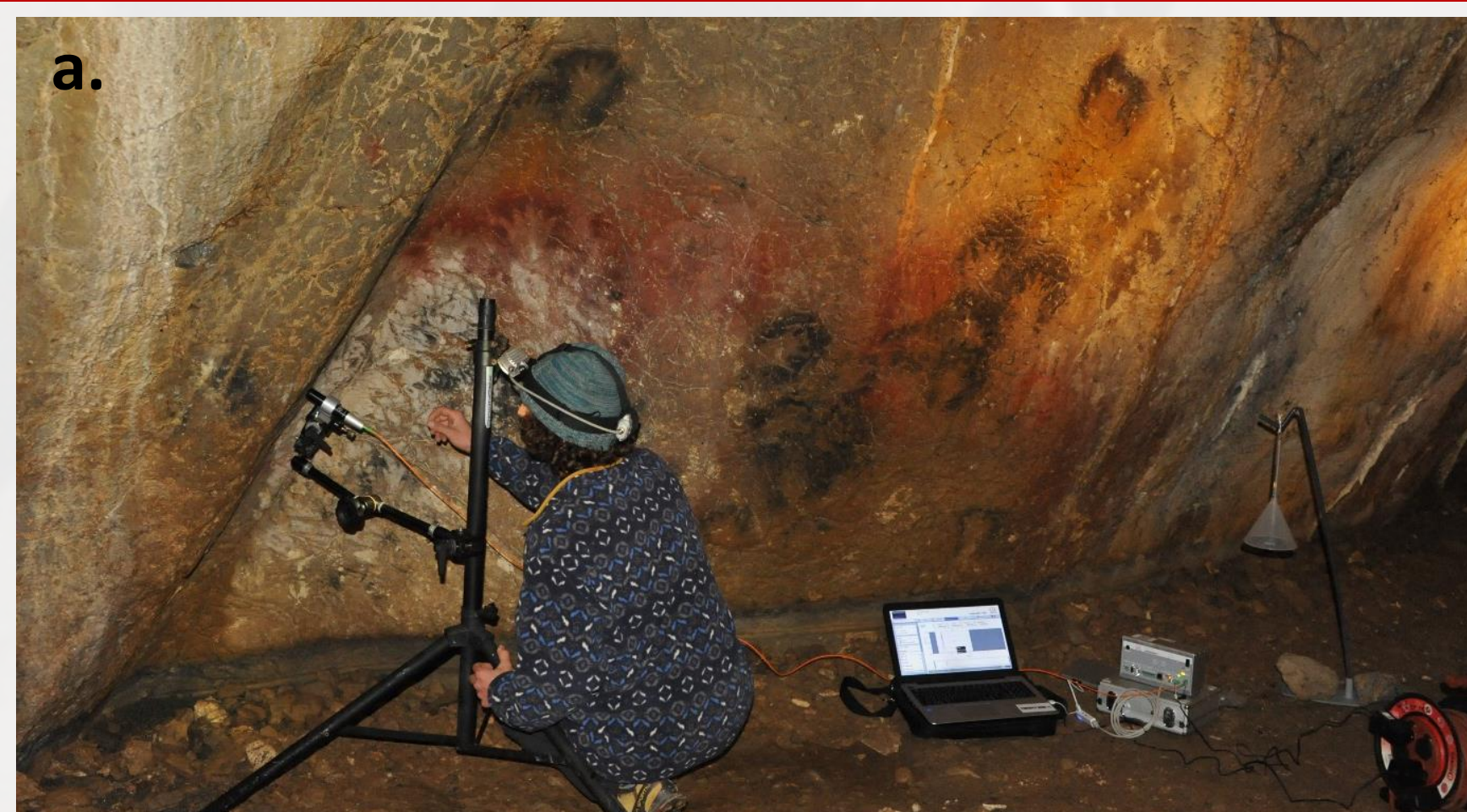
Figure.5 | Photo a. Device used to measure the water film on the “Grande paroi des mains”.
